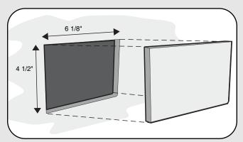
Cut a hole in the wall measuring 6 1/8" wide by 4 1/2" high.
